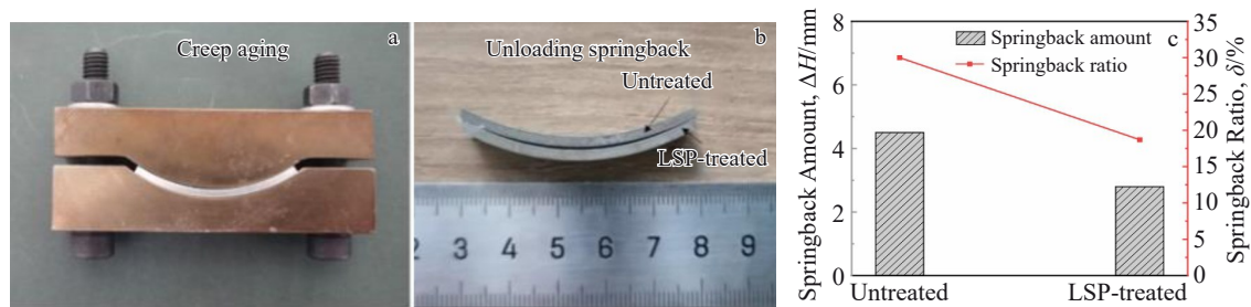
Fig.13 Creep aging device (a); untreated and LSP-treated specimens after unloading (b); comparison of springback amount and springback ratio between untreated and LSP-treated specimens (c)
