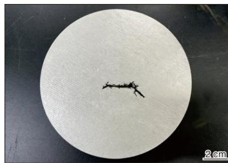
图 10 TC4 钛合金棒材缺陷的宏观形貌 Fig.10 Macrostructure of defect in TC4 titanium alloy bar
